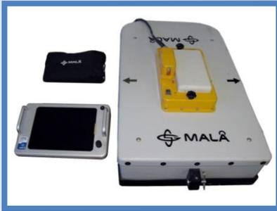
**Electronic tomograph-geoscanning system** is designed for carrying out geodesic, topographic, land-surveying and prospecting operations, as well as for carrying out different types of monitoring and scientific studies, such as quality studying the earth surface.
