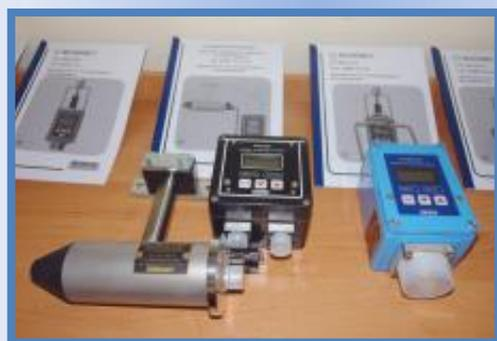
Methane thermo-catalytic sensor 0 ... 5% SH4;
