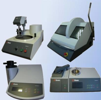
**Laboratory complex for the preparation of samples for metallographic analysis**
