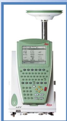
**GPS System 1200** is designed to measure distances, horizontal and vertical angles and exceeding in the implementation of topographic and geodetic works tachometric surveys, construction, layout, monitoring, and for applications of geodetic problems.
