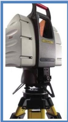
**Electronic laser 3D scanner** is designed for forming and supporting digital models of open pits and mines, determining the volumes of mining workings, storehouses, dumps, controlling mining operations, etc.
