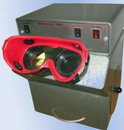
Luminescent set (Luminoscope LRV-1) used for determining the presence and the character of bituminous matter distribution in mining rocks (core, slime) and in capillary infusions.
